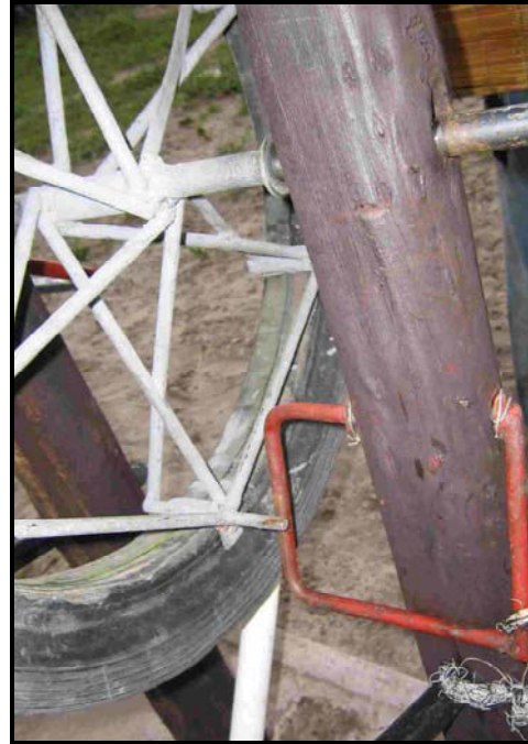
Figure 5.3 Photo of pulley wheel braking system. Pegs (grey) on pulley wheel make contact with the brake (red).
