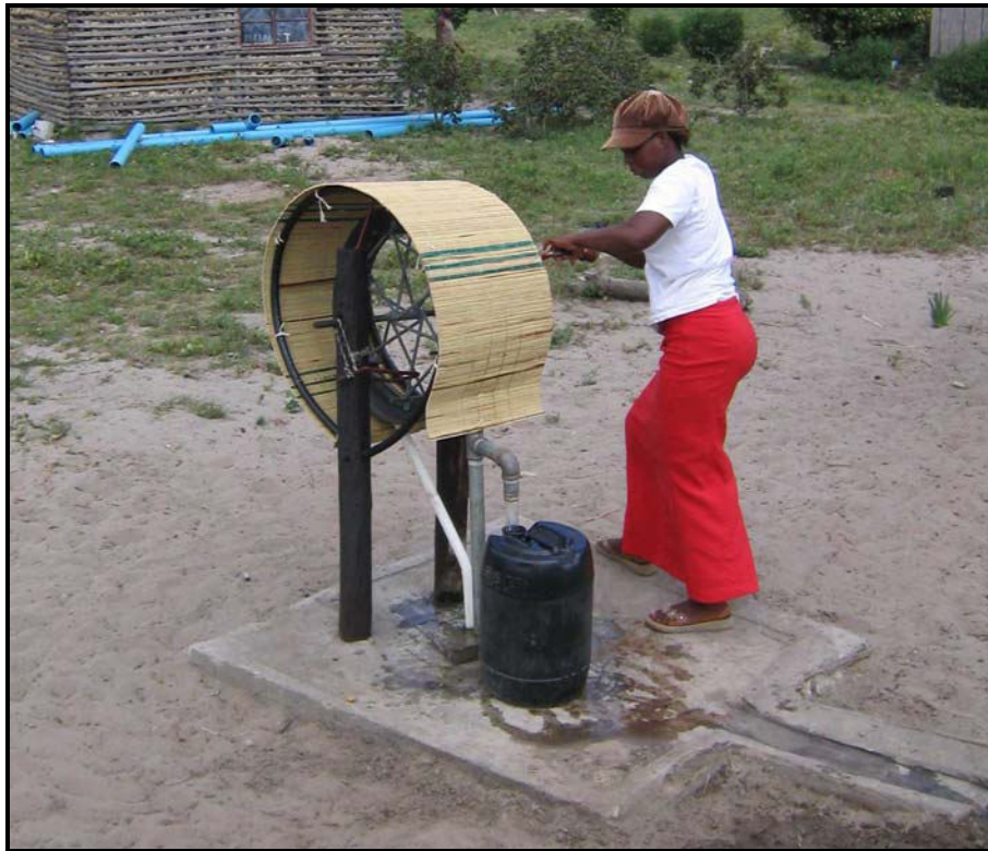
Figure 5.12 Photo of final project design of the R & W Pump in use (Thwala Pump)
