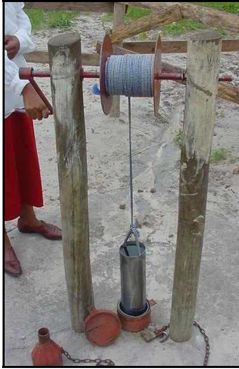
Figure 2. 4 Bucket Pump being lowered into tubewell
