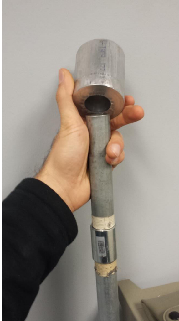
Figure 24. Top Buffer Pipe and Drive Cap for Exposed-Screen System A
