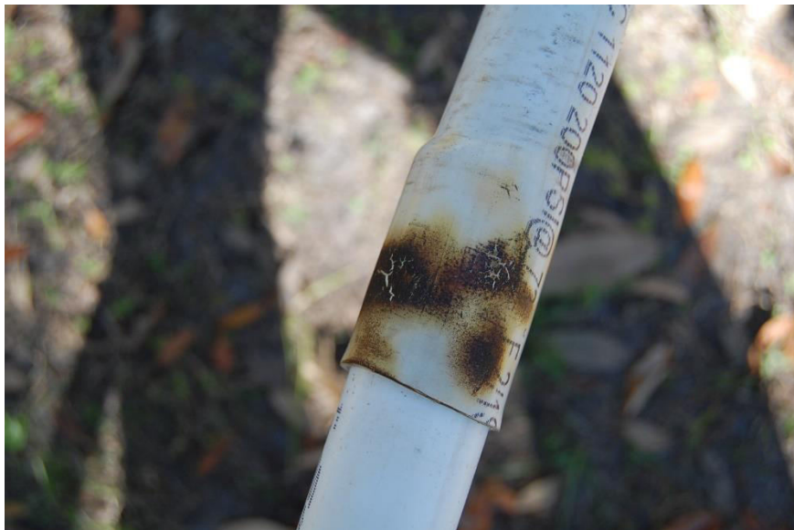
Figure 11. Final Result of Belling-Out a PVC Pipe
