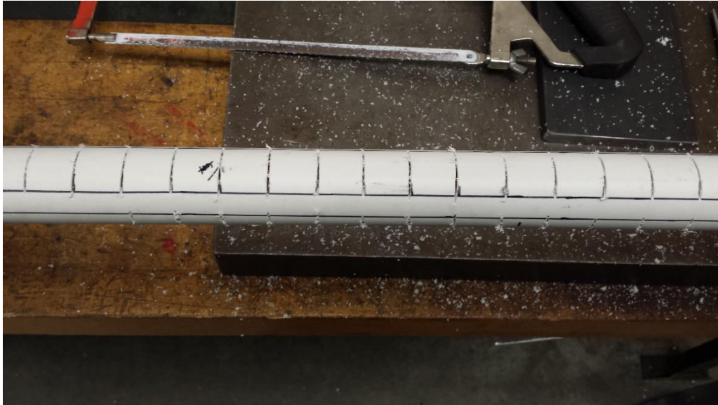
Figure 13. First Method of Screen Cutting
