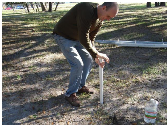
Figure 17. Example of Coring
