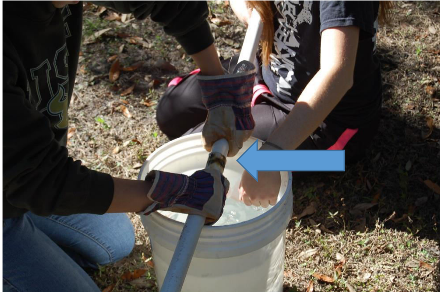
Figure 10. Belling Out a PVC Pipe
