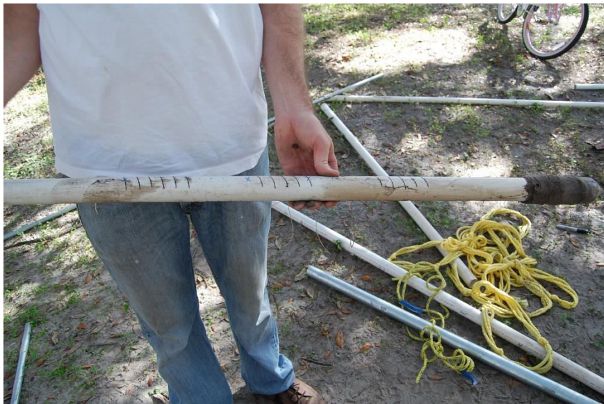
Figure 39. Sleeve Pulled Down on the Belled-End
