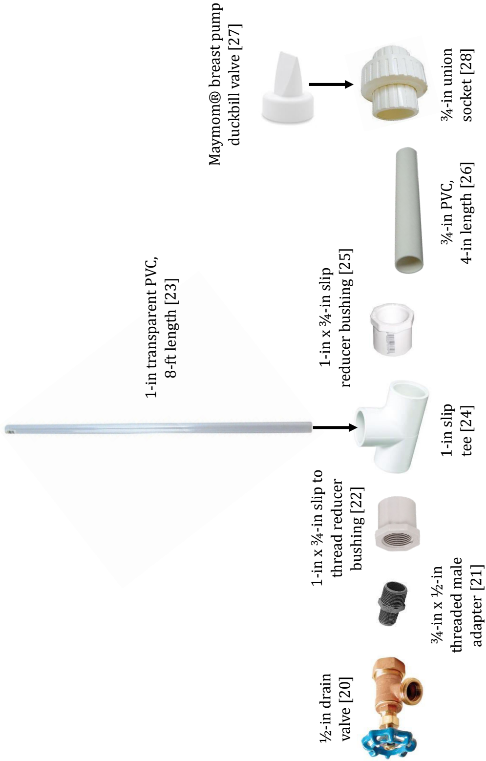
Figure A1. Detailed Maymom® breast pump duckbill valve manometer configuration (half of full manometer)
