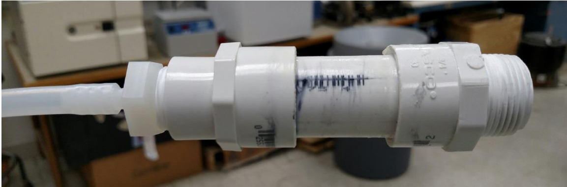
Figure 17. Vacuum pump connection
