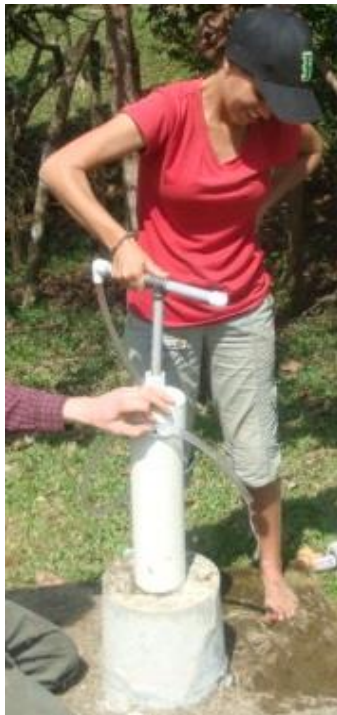
Figure 8: EMAS Hand Pump in Operation
