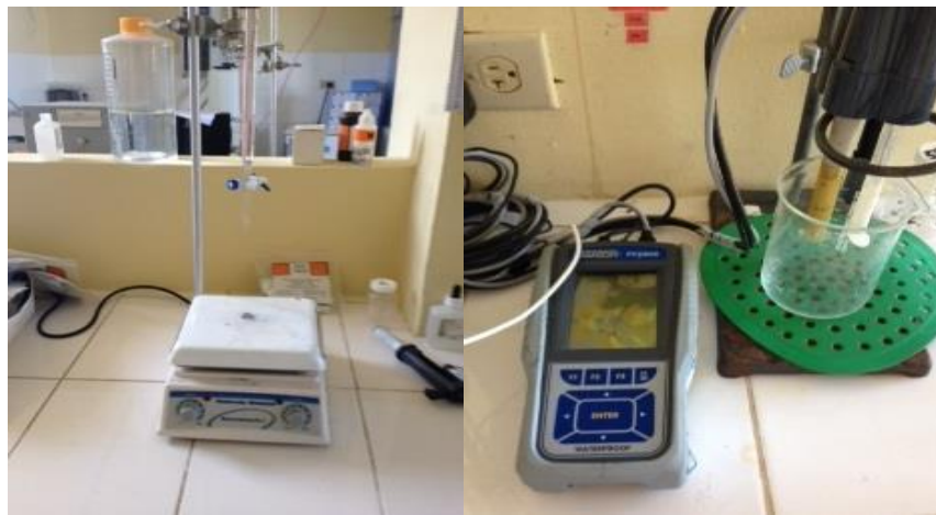
Figure D.6: (a) Alkalinity Titration Apparatus (b) OAKTON PCD 650 Probe
